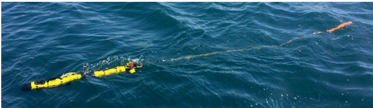
Figure 2. Marine Magnetics Explorer magnetometer towed behind the Iver3 AUV.
