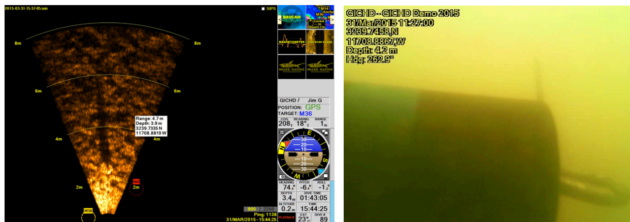
Figure 18. Left: Screen capture of Navigator's scanning sonar ensonifying a simulated ERW target. Prominent shadow is cast behind (above in image) the target. Right: Screen capture of simulated ERW target from Navigator's video recorder.
