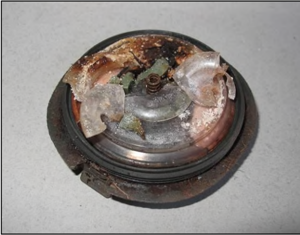
Even when rusted, the steel springs had lost little of their original mass (SB-33 left, SB-81 right)
