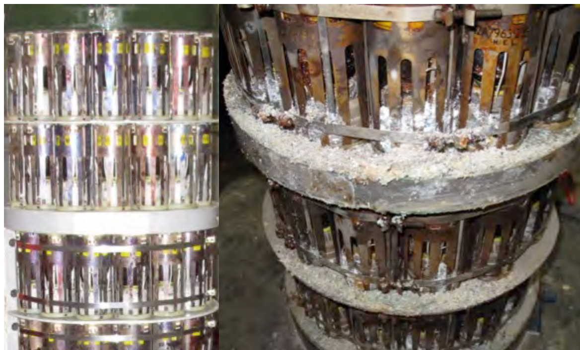
Figure 4: BL755 cluster bomb submunitions of the same age from the same stockpile. Some (on the left) have been kept dry and remain in good condition; others (on the right) were subject to flooding and suffered severe corrosion.
