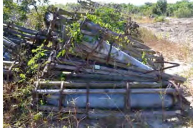
Abandoned S24 rockets in northern Mozambique containing rocket propellant in which the stabilisation compound is likely to have degraded, leaving weapons that are unstable and potentially liable to auto-ignition.
