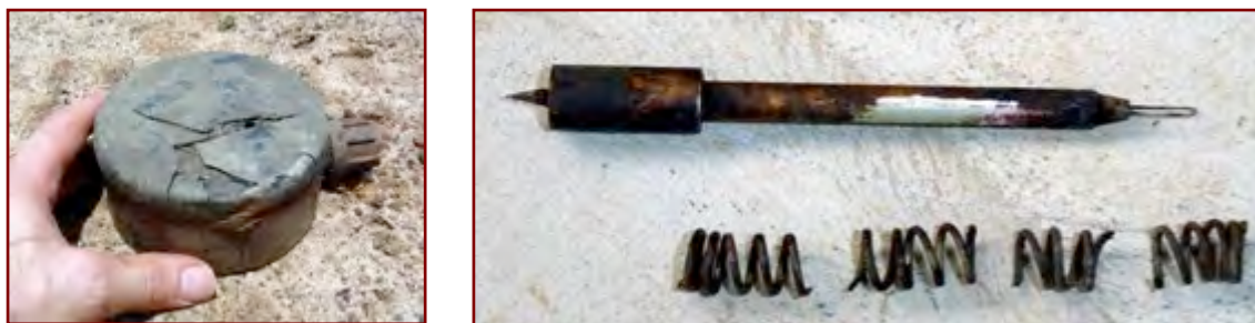
Figure 9: PMN from Cambodia showing cracked and damaged rubber external casing and rusted striker spring
