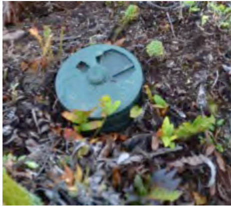
Surface laid P4B anti-personnel mine showing the effects of thirty years exposure to UV light, rain, wind, snow and temperature cycles, in the Falkland Islands/Malvinas.
