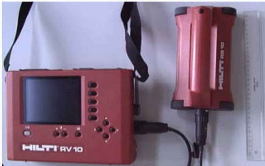
Figure 7.5: Ferrosan RV 10 monitor (left) and RS 10 scanner (right) (ruler length: 30 cm)
