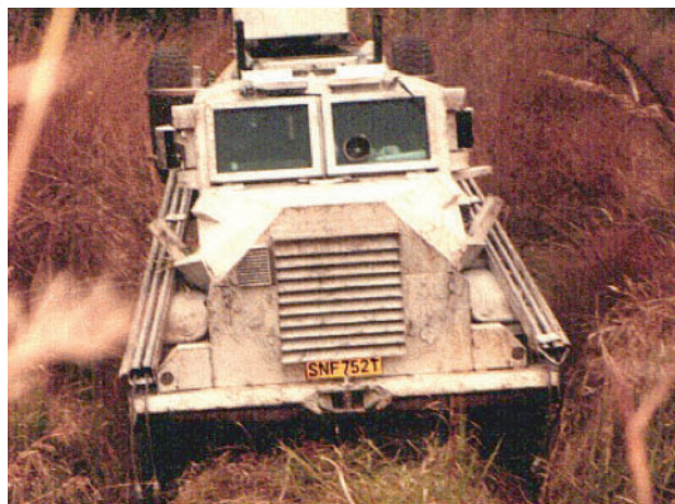
Casspir with suction tubes during sampling of power lines in Mozambique (Mechem, early 90s)
