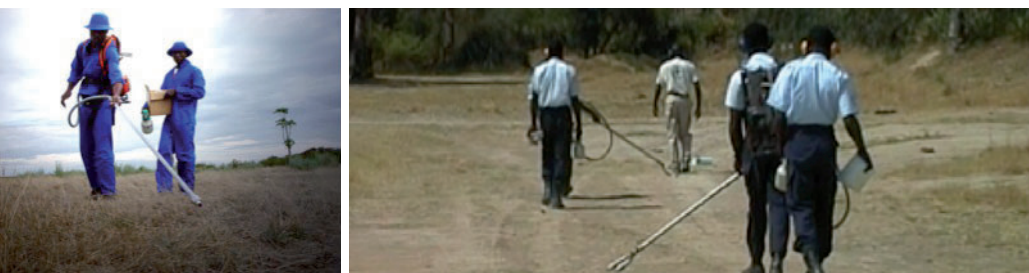
Left Petrol driven suction units have been the preferred system, but battery or gas driven prototypes have shown promising results Right A sampling team walking in the tracks of a Casspir vehicle in Angola
