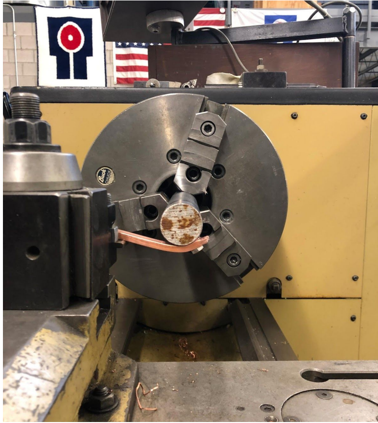
Figure 10: End view of the lathe and coil being wrapped
