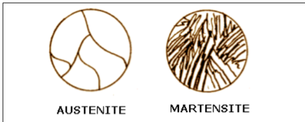
Figure 3 : Molecular steel before and after Quench Heat Treatment
