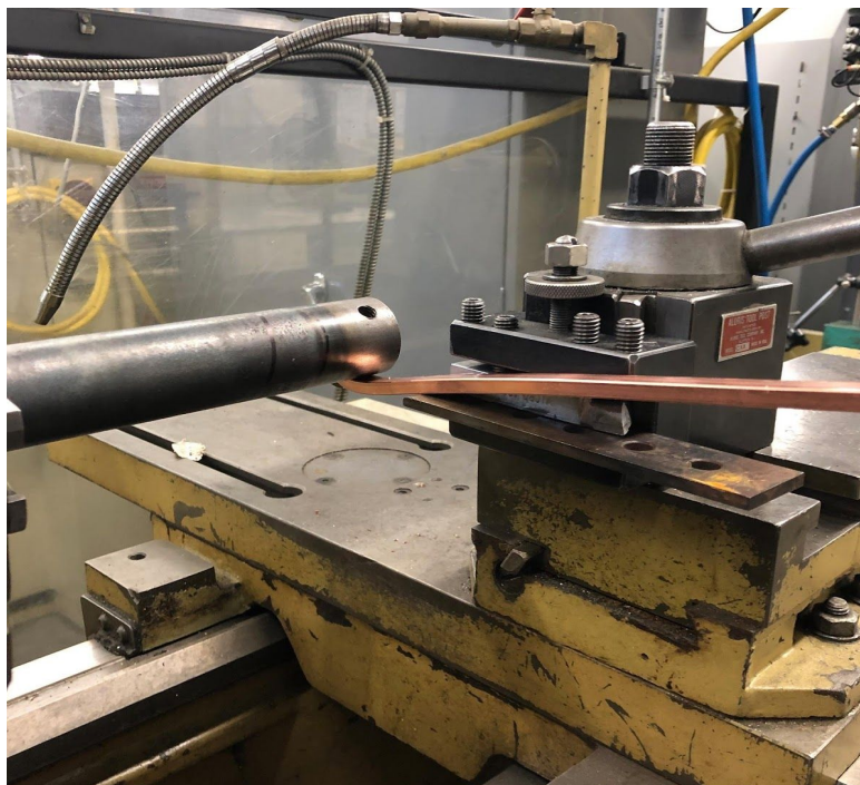
Figure 9: The copper tubing ready to wrap on the lathe
