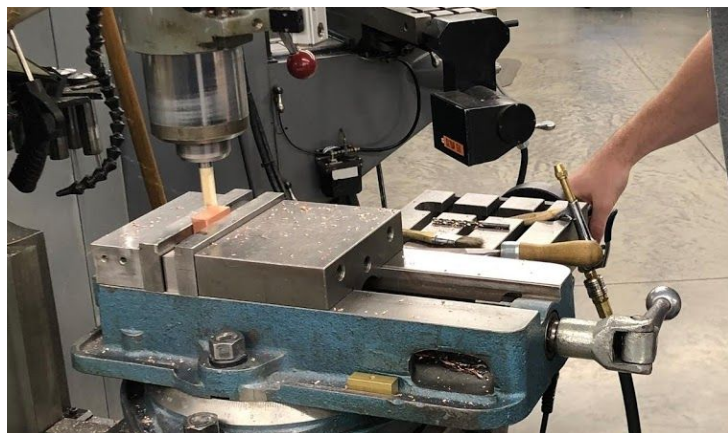
Figure 12: Machining a copper block for a strong connection
