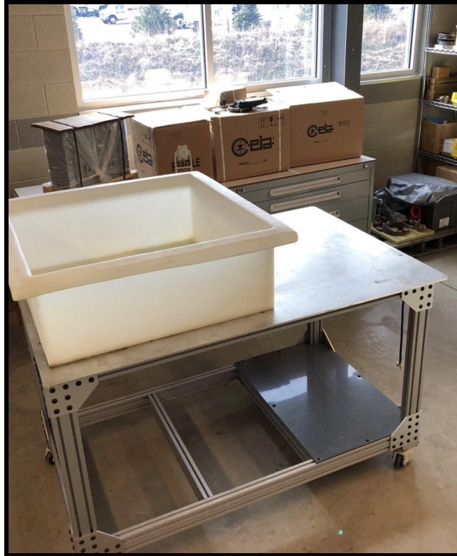
Figure 5: Tub and aluminum stand on locking casters
