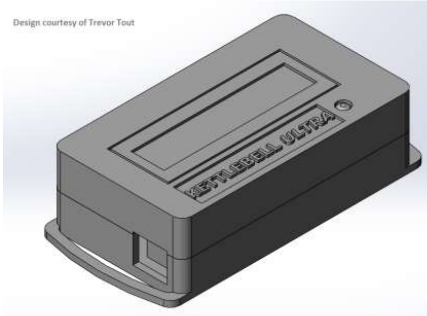
Figure 67: Housing Design for Secondary Board
