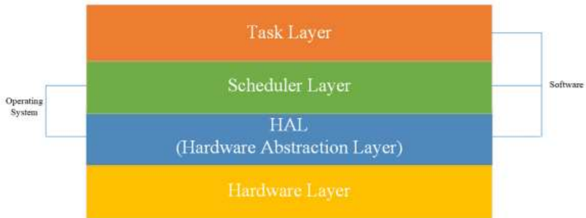
Figure 73: The diagram showing the different levels of the embedded software architecture.
