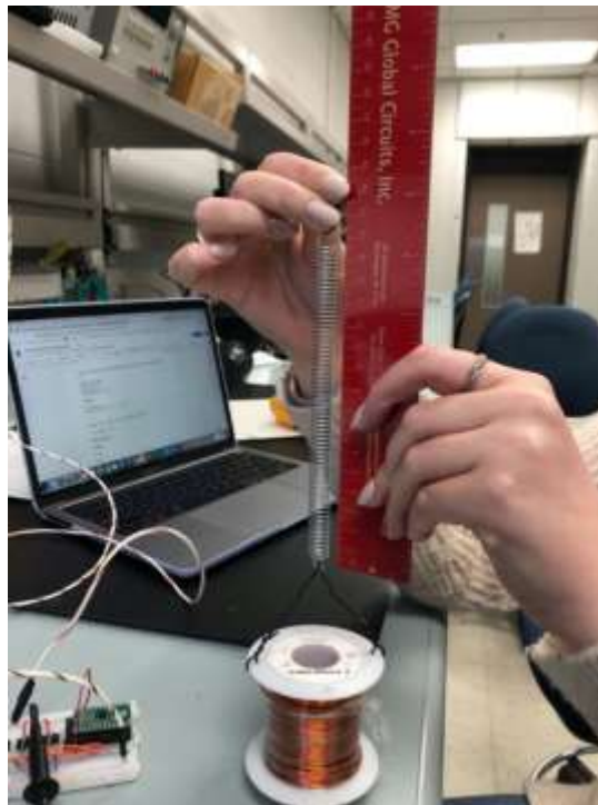
Figure 14: The setup to determine the spring constant of the spring in use.
