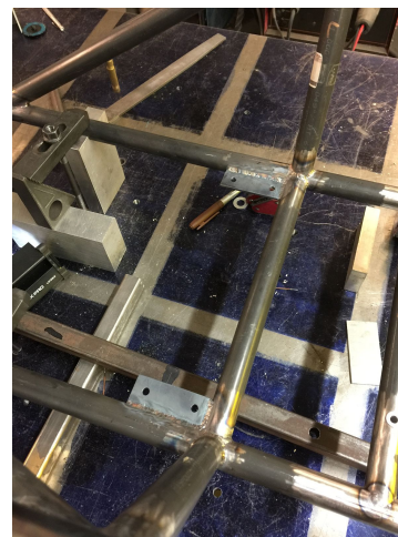
Figures 33, 34, and 35: T-Bar Design, Measuring the T-Bar, Mounting Plates Welded to Frame
