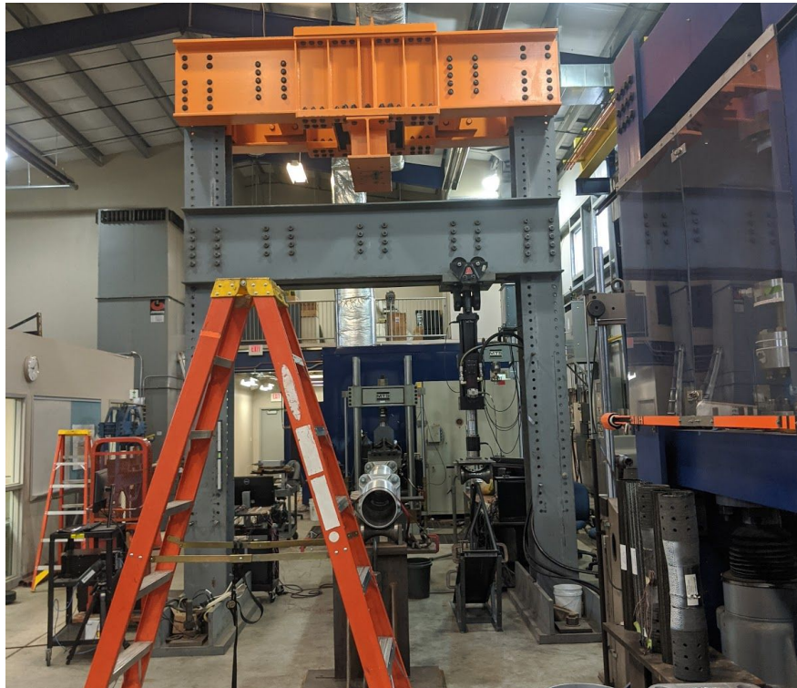
Figure 12: The 300Kip Press in the Gas Turbine Testing Facility
