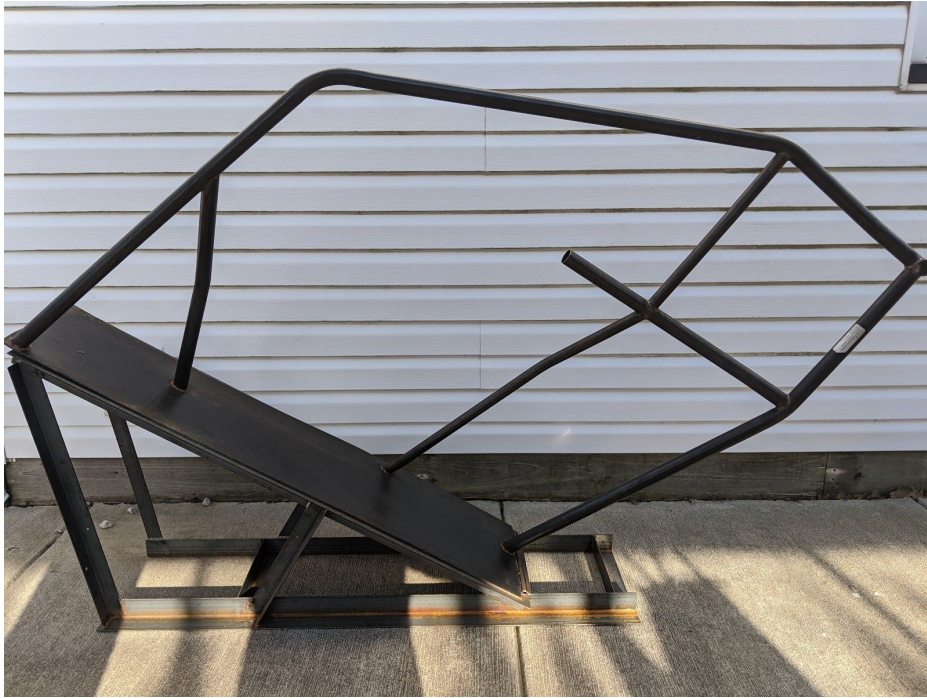
Figure 14: Front Tube Frame After Test
