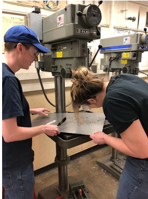
Figure 10c. Drilling sheet metal for hopper
