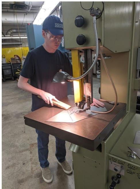
Figure 10b. Cutting sheet metal for hopper
