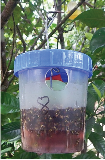
Figure 1. Male lure trap crafted from urine sample cup used in the 2014 survey.
