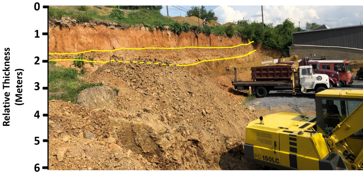
Figure 1.2. Interpreted channel outcrop at Paleochannel site location
