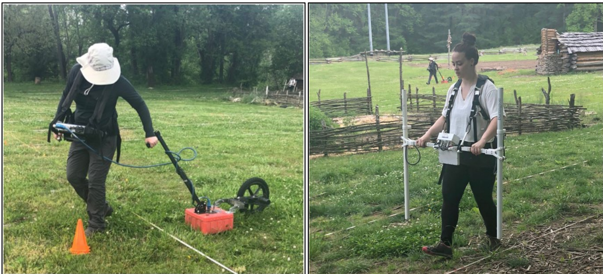
Figure 2.7. Geophysical Instruments used for this project included: (left) a GSSI SIR4000 GPR control unit with a 400 MHz antenna and survey wheel and (right) a Bartington Grad 601-2 dual fluxgate magnetic gradiometer.
