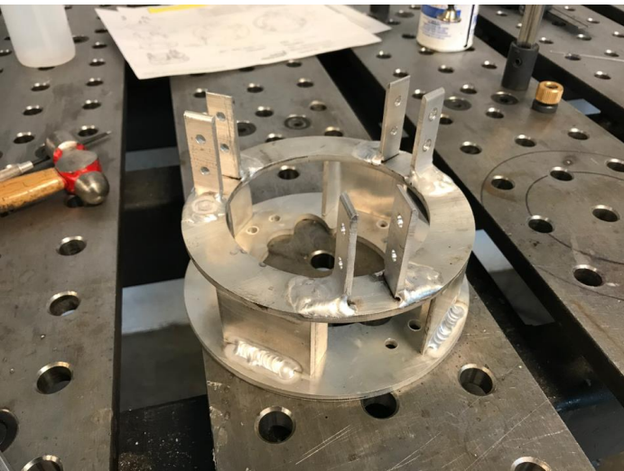
Engine Mount - Post Weld
