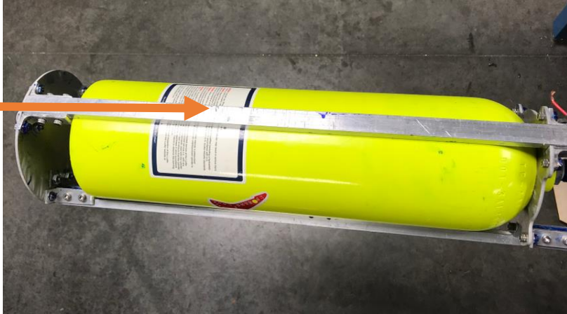
Pressurant Gas Storage
