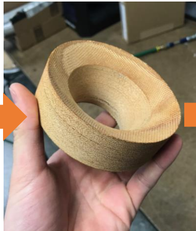
Throat insert ready for silica wrap
