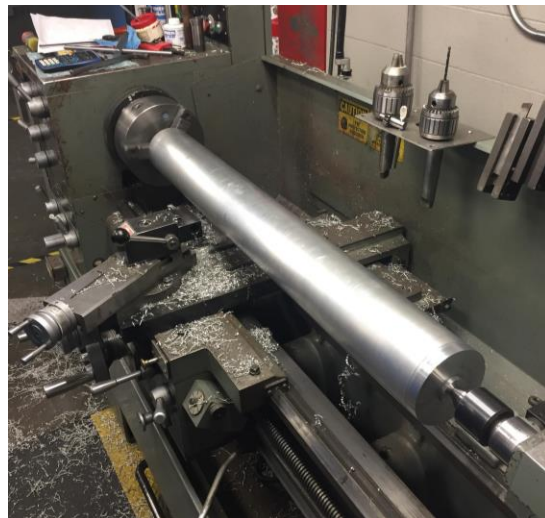
LOX (top) & Fuel (bottom) tank main bodies on lathe
