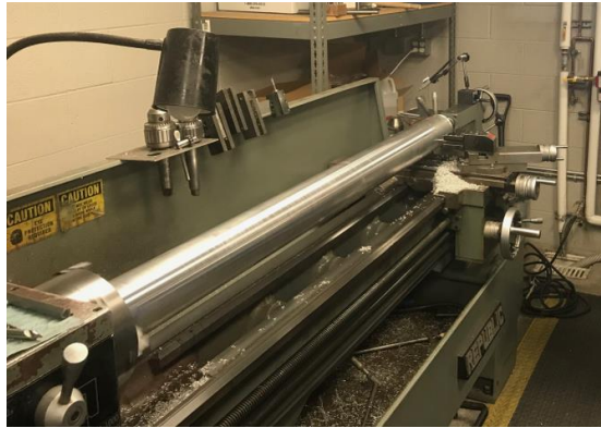
LOX (top) & Fuel (bottom) tank main bodies on lathe
