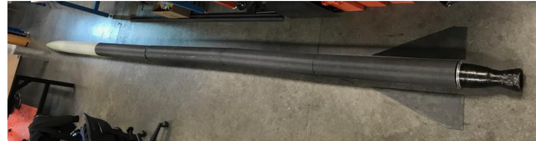
5 lower layer segments with nose cone, fins, & engine
