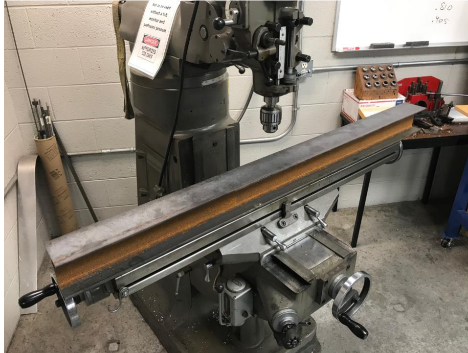
I-beam support holes being drilled
