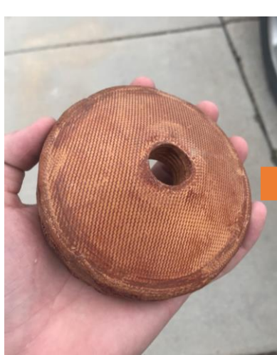
Blank silica-phenolic throat insert
