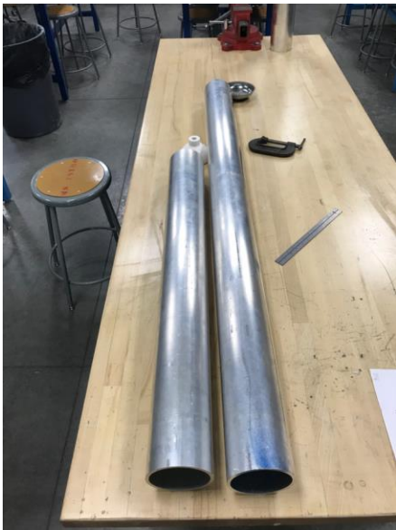
Tank main bodies after being cut to length
