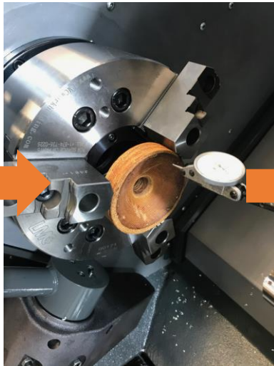
Machining the throat contour
