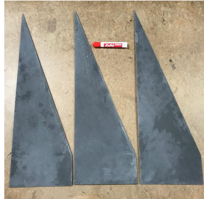
3 fin cores of aft swept leading-edge trapezoid shape
