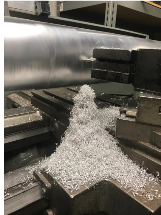
Turning OD of LOx Tank
