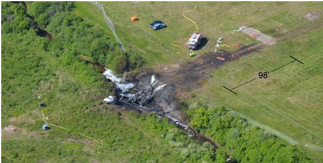
Figure 2. N121JM Runway over run showing distance from ALS/localizer to perimeter fence
