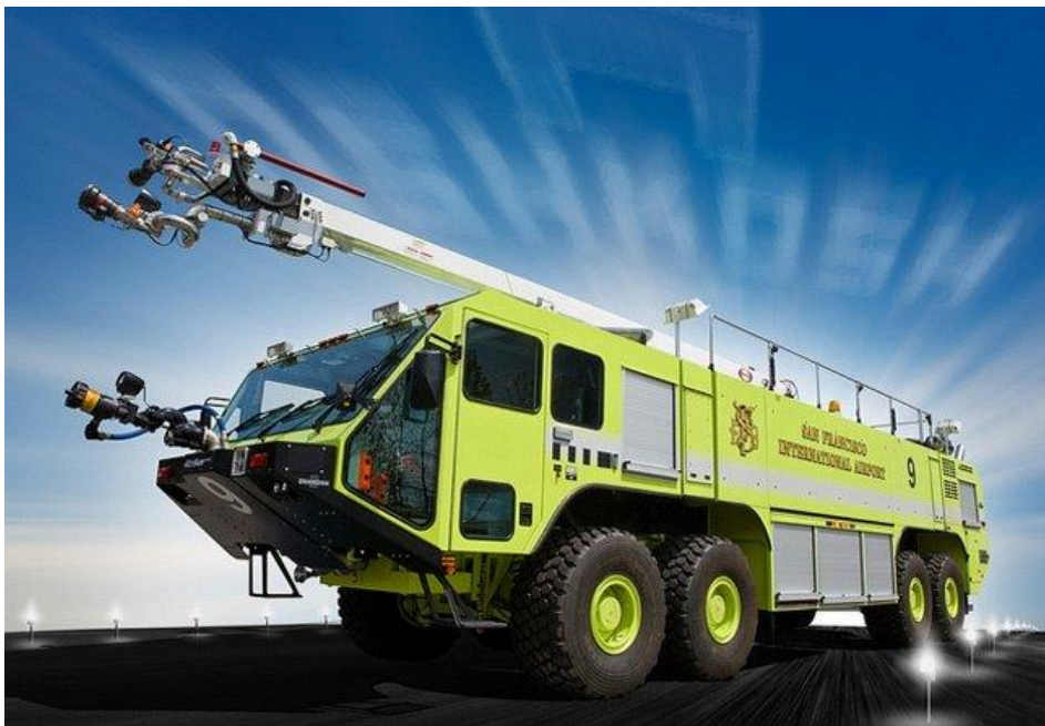
Figure 20. Oshkosh Striker 4500 (Rescue 9) Exhibit Photos. Equipped with the high-reach extendable turret (HRET) and piercing nozzle. Source, Oshkosh Corporation.
