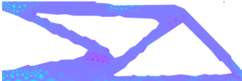
Figure 6.11. The optimal topology of a 1 by 3 cantilever plate under concentrated load at the tip (Wang et al., 2003)
