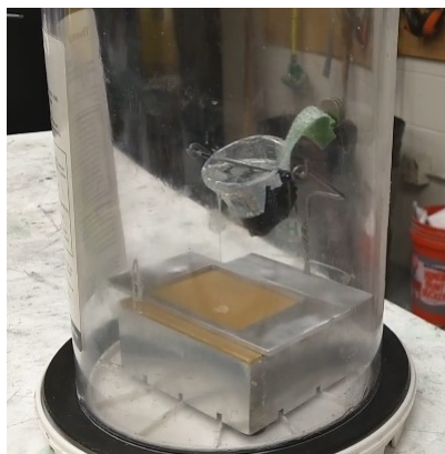
Figure 3.2 The vacuum chamber apparatus used for casting of micro-pillar arrays.
