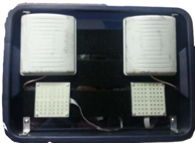
Figure 4-1 Antenna board installation for sleep disorder monitoring.
