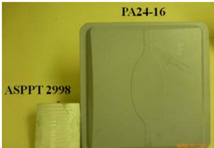
Figure 2-3 PA24-16 ( 29 \times 29 \times 2.5 \text{ cm}^3 ) and ASPPT 2998 ( 10.5 \times 10 \times 4 \text{ cm}^3 ) radar .The figure shows the size difference between two radars [44].
