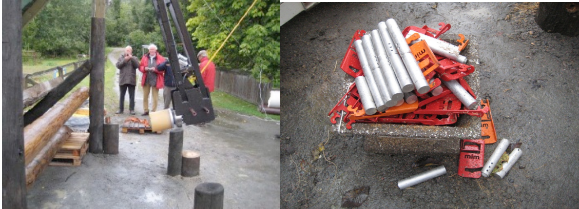
Figure 6.4 (left) 2011 Sweden Comparison Testing Using the MiM Pendulum Tester (Right) Collection of used and unused frangible pins and MiM clips.
