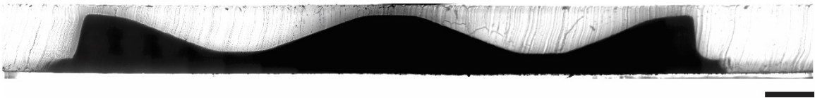
Figure 4.12 Cross-section of PDMS casting made from SU-8/glass waveform mold. Scale bar: 1 mm.
