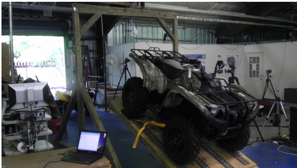
Figure 3.1 ATV and tilt platform inclined to pitch angle of 25 degrees declination relative to the horizontal.
