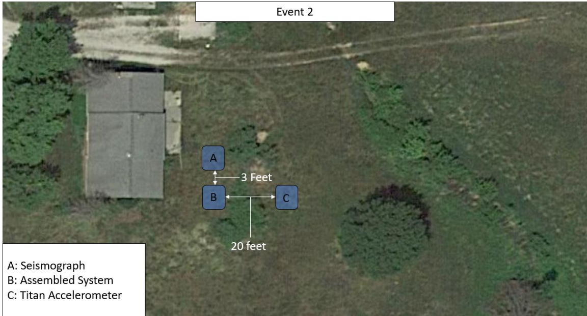
Figure 4.14: Event 2 Map of Installed Monitoring Systems
