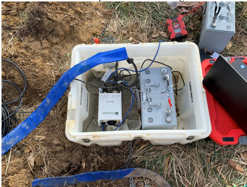
Figure 4.12: Data Logger Connection to Titan Accelerometer
