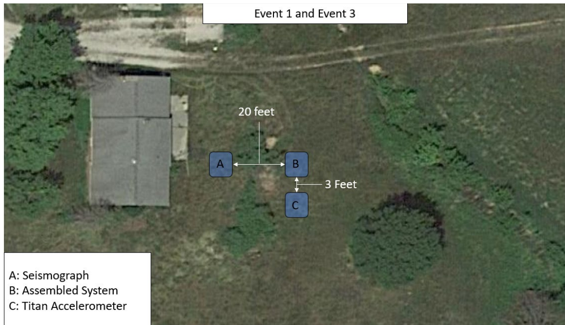
Figure 4.13: Event 1 and Event 3 Map of Installed Monitoring Systems
