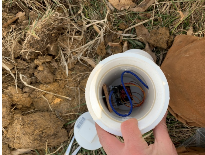
Figure 4.5: Electronic Positioning within the PVC Housing
