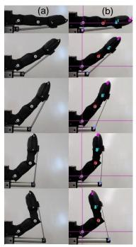
Figure 3.1 (a-b) Incremental extension of the linear actuator. (b) The placement of tracking markers in Tracker.
