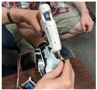
Figure 4.12 The steel strip for the thumb being fixed to the thimble.
