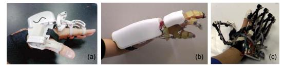
Figure 1.3 Examples of high- and low-profile rigid linkages used in orthoses that were designed by (a) Wang, et al. [16], (b) Hasegawa, et al. [17], and (c) Ben-Tzvi, et al. [18].
