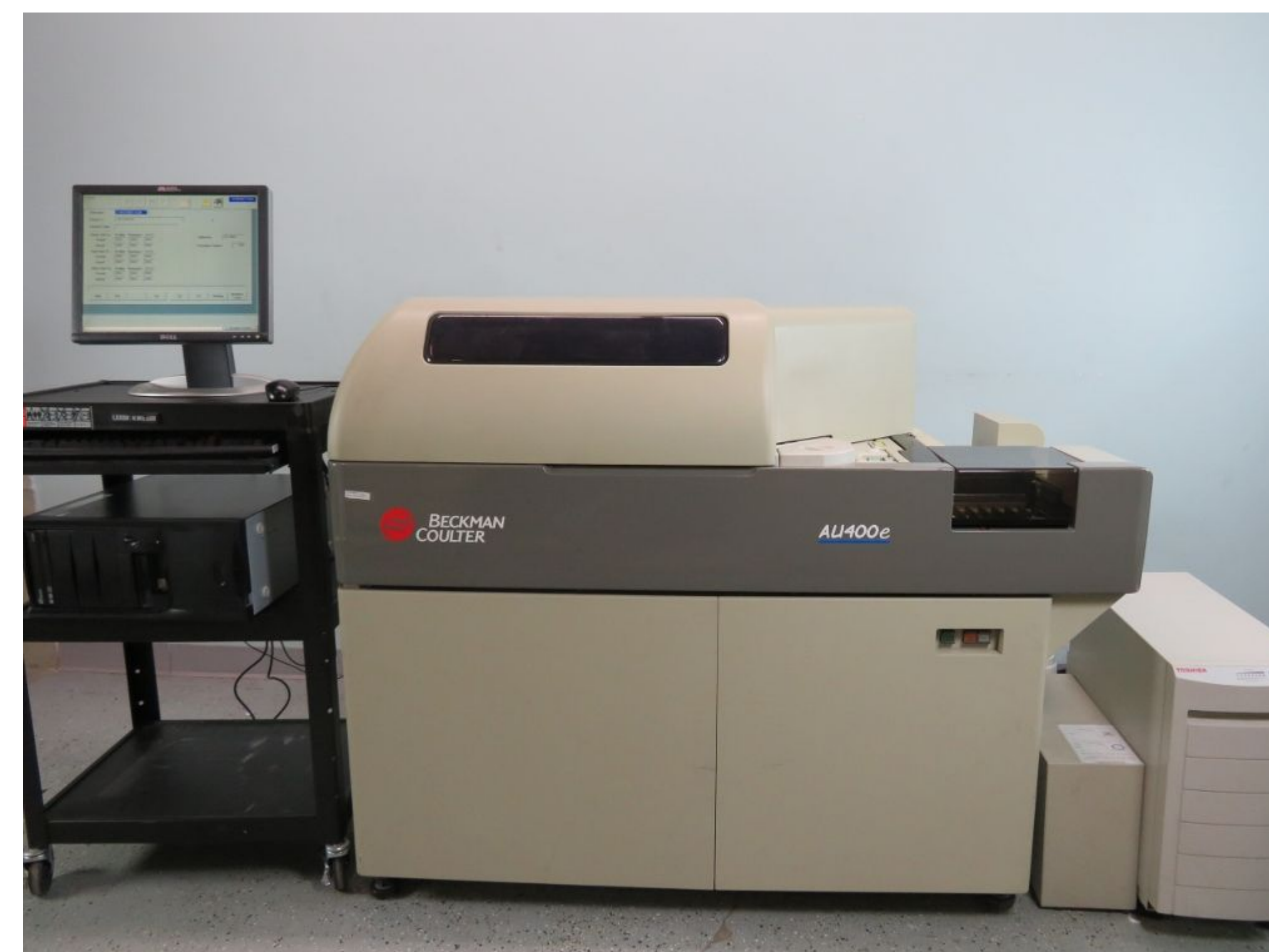
Figure 2: The Beckman-Coulter AU400e Analyzer. As a blood serum diagnostics we require this machine in order to do assays. Since our kit uses capillary blood rather than venous blood we have to do comparative studies to prove that the results between those two are the same or similar enough to be used in place of the other. Another study that needs to be done is a "stability" test due to the fact that our service involves sending blood through the mail, we need to make sure that the analytes in the serum can survive the journey and the temperatures it will encounter. We are comparing our values to those of other established companies in order to show that our method works.
