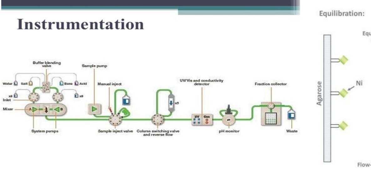
Fig. 4. Instrumentation of fast-protein liquid chromatography (4).
