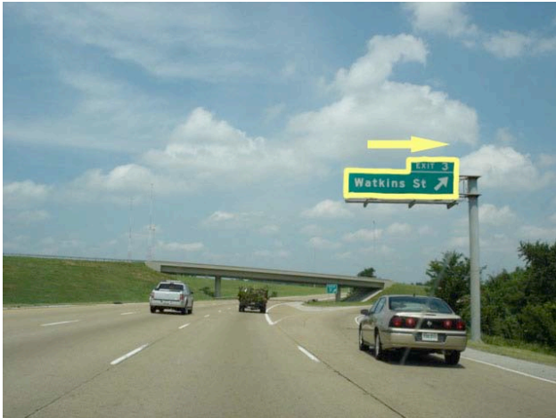
Figure 7: A driver following a highlighted exit sign. Note that all other AR components not in the driver's line of sight has disappeared.
