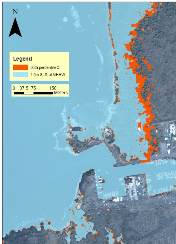
Figure 7: Example of map showing inundation and error polygons north of Honokohau Harbor at Kaloko Honokohau National Historical Park. There is little uncertainty in steep areas such as walled areas within the Harbor and cliffs south of the Harbor. There is greater uncertainty illustrated by wider 95 th percentile confidence interval bands in areas with gradually sloping land surfaces such as the area behind Aiopio Fishtrap.
