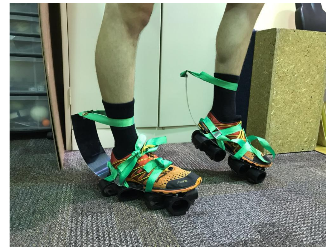
Figure 1. The original ankle-based design created by research team in 2018.
