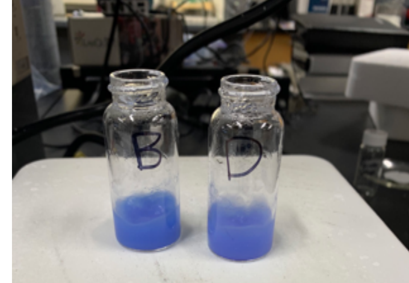
Figure 2. Zeolite-thionine suspension after boiling and cooling.
