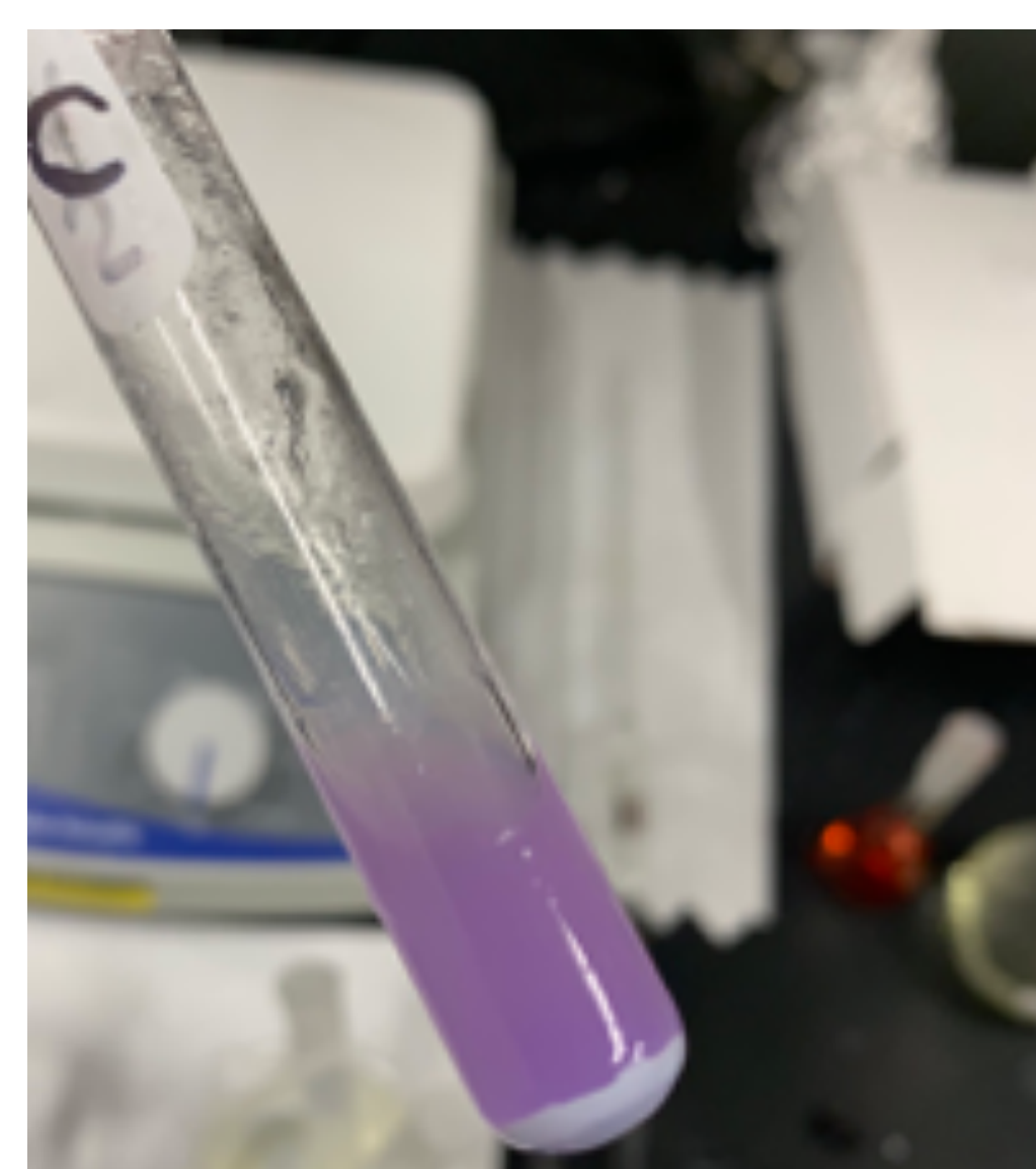
Figure 3. Bad batch of zeolite in a Zeolite-thionine suspension after boiling and cooling.
