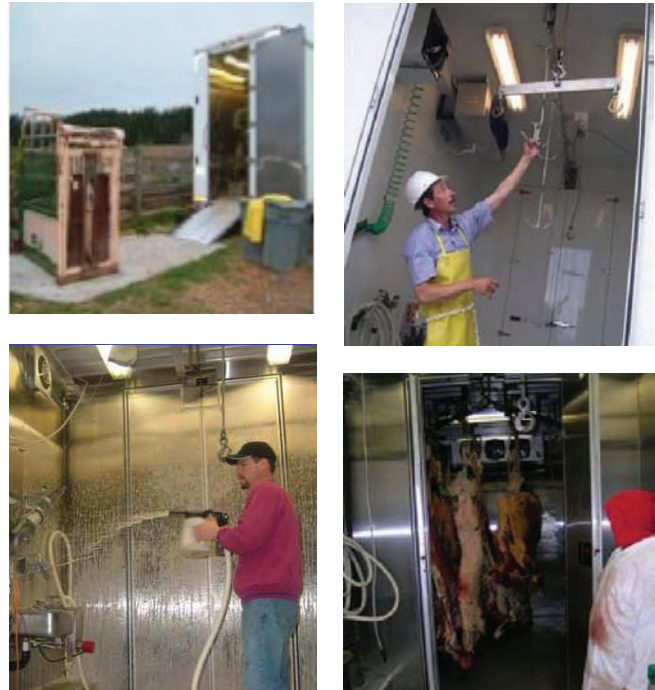
Figure 6. The general process of a mobile slaughter-type operation (clockwise from top left): Animals are restrained outside the unit and stunned; brought into the unit with a winch; the trailer door is closed, animals are minimally processed into halves and stored in the middle of the unit; the rear of the unit is cleaned, then the process begins again with the next animal.
