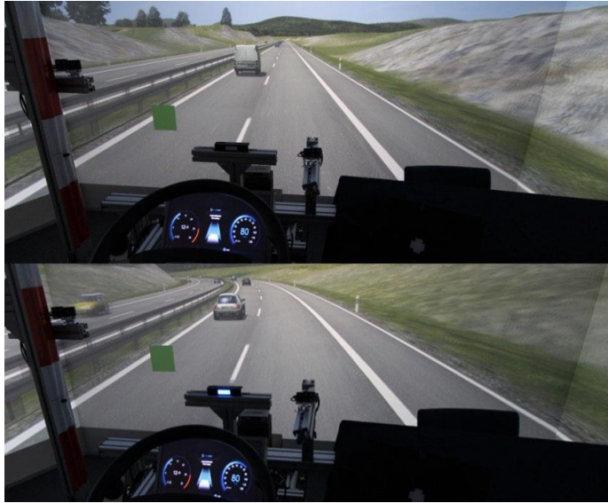
Figure 1. Top: peripheral vigilance task (PVT) in the L2 condition. Bottom: PVT in the L3 condition with the take-over LED near the steering wheel.
