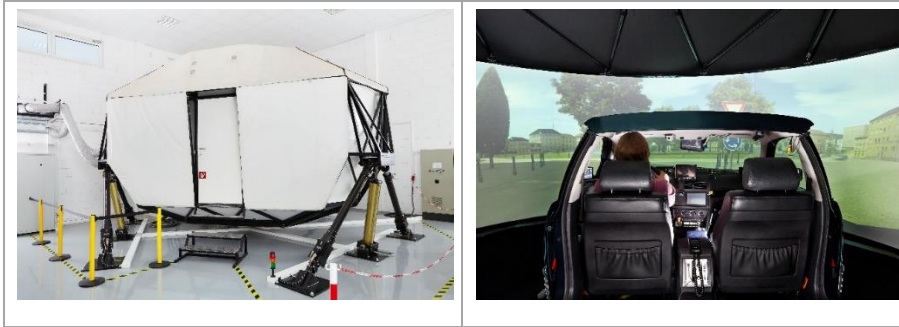
Figure 1: High-fidelity motion-base driving simulator from the outside (left) and from the inside (right)
