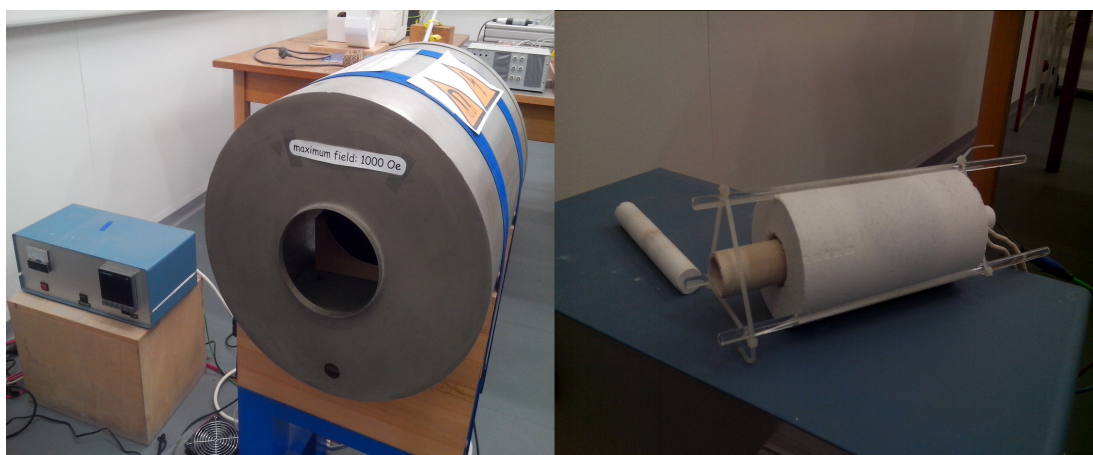
Figure 1.4: Magnetically shielded AF/ARM coil with temperature control unit and fan (not in place) (left) and high temperature insert (right).
