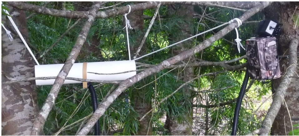
Figure 3. Bait station setup, with tube, trigger, cable, and camera assembly installed within vegetation on the island of Guam, USA, during 2015 and 2016.
