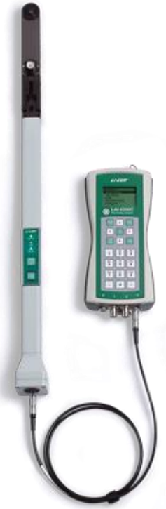
Figure 2.7. LAI-2200C Plant Canopy Analyzer (optical sensor, left; console, right) (LI-COR Plant Canopy Analyzer Manual, 2016).
