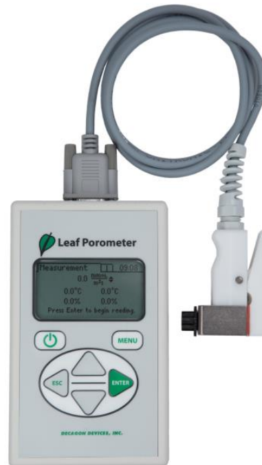
Figure 2.6. Leaf porometer used in this experiment (Decagon Device Inc. Leaf Porometer Manual, 2016).
