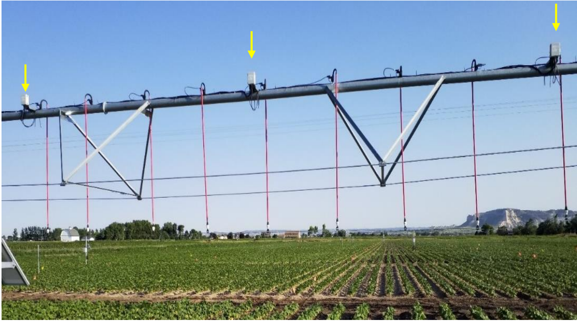
Figure 1.7. Solenoids, drops, and nozzles of variable rate irrigation (VRI) system and wireless control nodes (white boxes pointed by yellow arrows).
