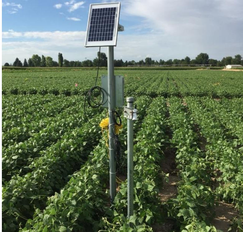
Figure 2.3. Set up for IRT located in the middle rows of an irrigation plot.
