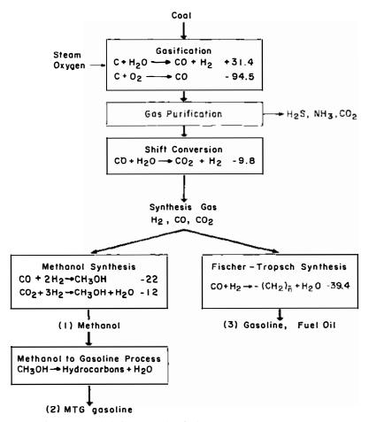
Figure 1 Process steps in indirect coal liquefaction.
