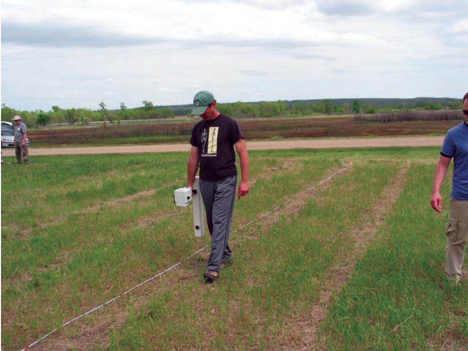
Figure 15. Participants practicing with the single fluxgate gradiometer at the Taylor Bluff site during the archeological prospection workshop (view to the east).
