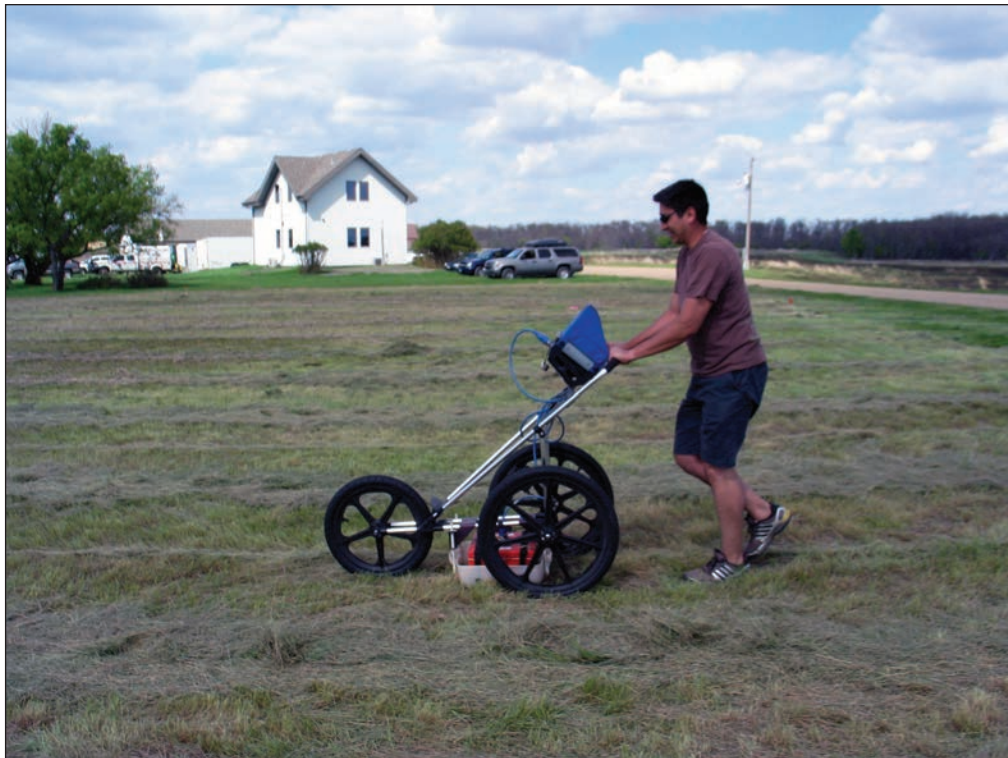
Figure 18. Conducting the ground penetrating radar survey with a GPR cart and 400 mHz antenna at the Taylor Bluff site (view to the northeast).
