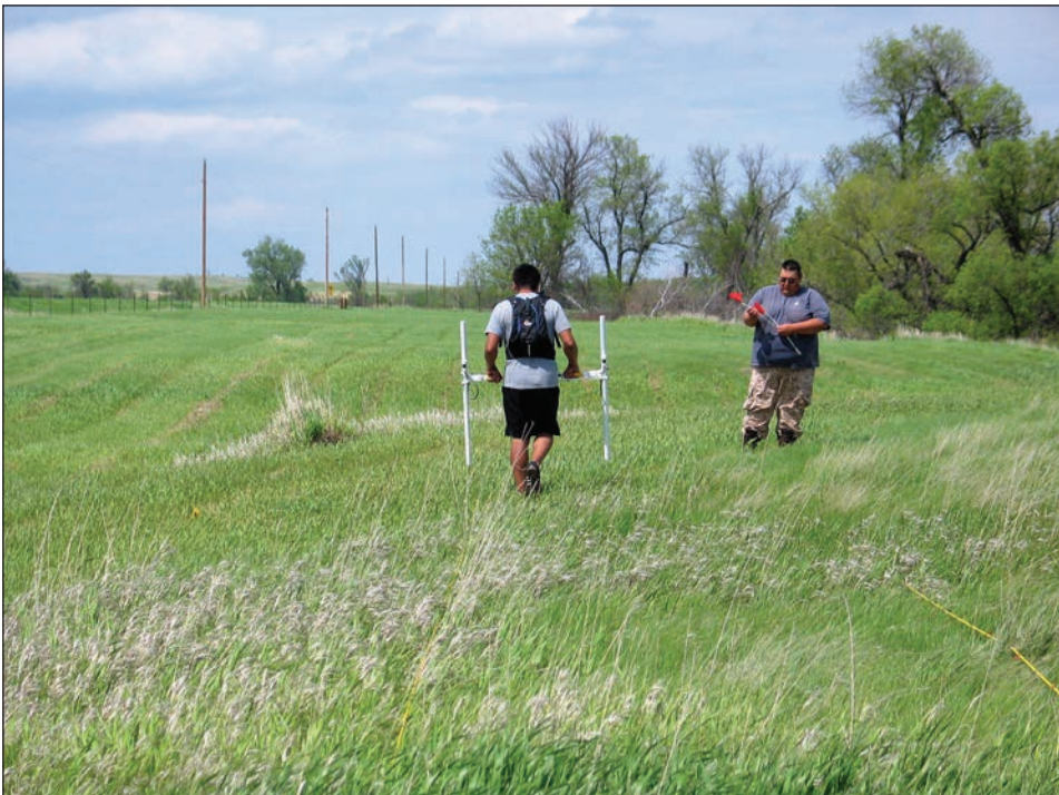
Figure 16. Conducting the magnetic survey with the dual fluxgate gradiometer at the Elbee site (view to the north).
