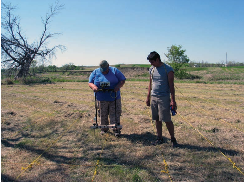
Figure 17. Conducting the resistance survey with the resistance meter and twin-probe array at Site 32ME2377 (view to the south).
