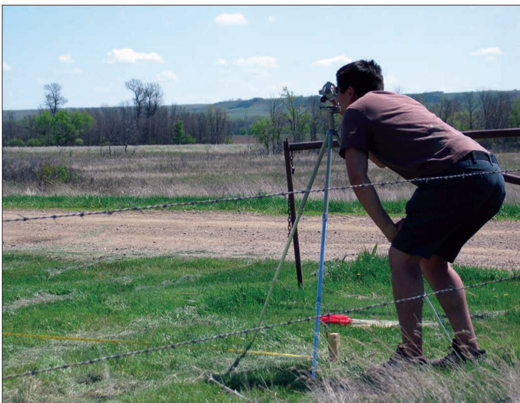
Figure 8. Using the surveying compass to set out the geophysical grid at the Taylor Bluff site (view to the northeast).
