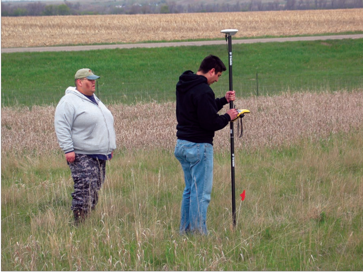
Figure 13. Mapping the grid corner stakes with the GPS unit at the Elbee site geophysical project area (view to the northwest).
