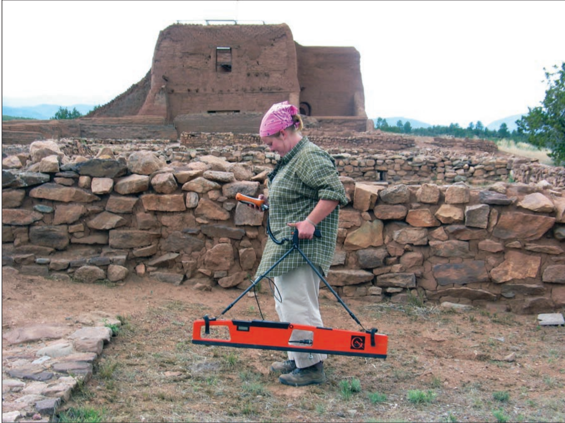
Figure 19. Demonstrating the use of the electromagnetic induction meter for conductivity surveying (view to the north).
