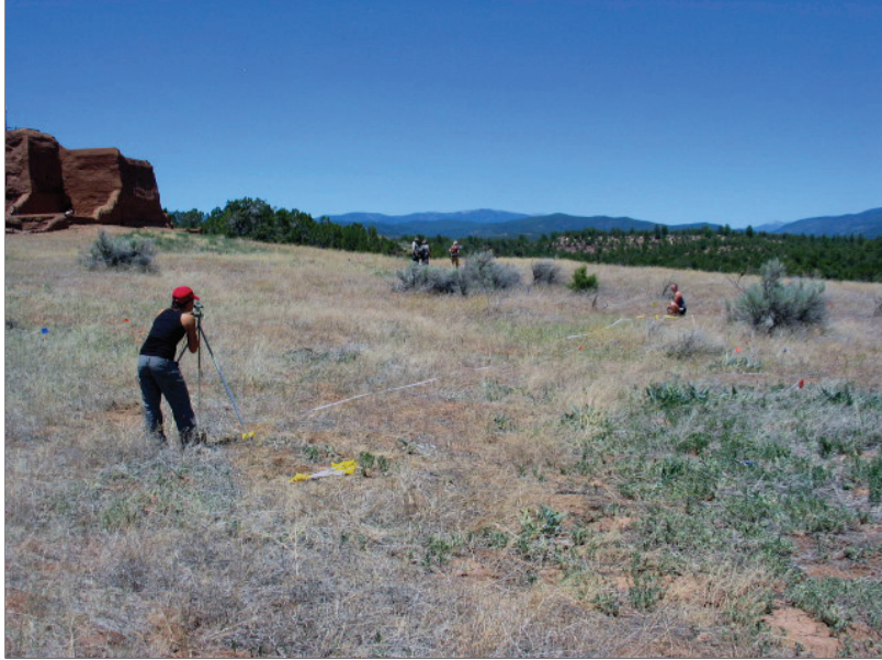
Figure 6. Laying out Area A with a surveying compass and 100-m tape (view to the northwest).
