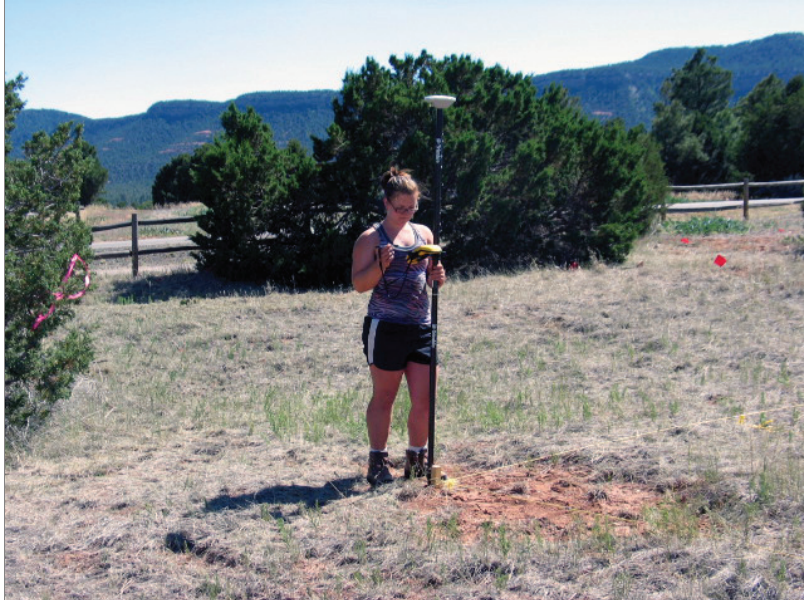
Figure 7. Collecting grid coordinate locational data with GPS unit and external antenna (view to the south southwest).
