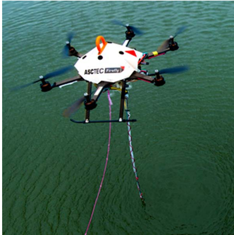
Figure 1. Photograph of the water sampling UAV in the field (not shown to participants).
