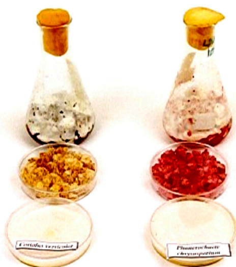
Figure 2. Growth of two white-rot fungi Phanerochaete chrysosporium and Coriolus versicolor in the fermentation of dye-adsorbed substrates. (Picture taken by author P. Nigam from lab experiment, not published anywhere).
