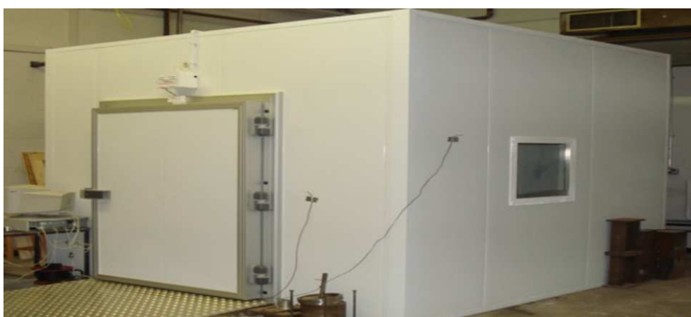
Figure 1: Climatic chamber used for testing the heat pump.
