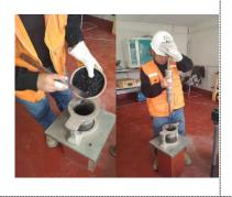
**Figure 6.** MAC is placed left fresh from the oven in the Marshall test specimens, which are struck an average of 75 times around the mold.
