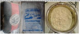
**Figure 3.** The filler has been selected according to its composition, lime and portland cement type I for being oxidants and silicas for being mineral with properties similar to lime [1].
