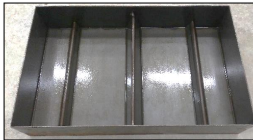
Figure 3. Norma ASTM C 1579 Metal Mold
