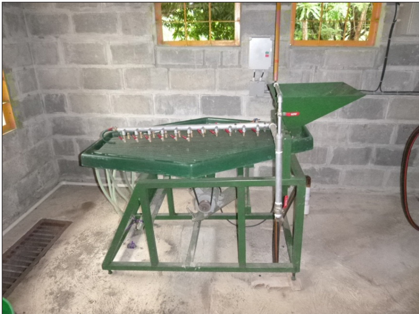
Figure 3. Carlos’ trommel for rough gravitational extraction.
