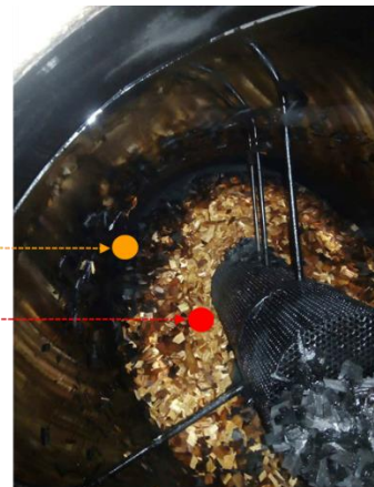
Figure 7.3: Difference on temperature and decomposition stages of the wood chips in a non-complete pyrolysis experiment. Red and yellow lines represent the evolution of the inner reactor (T01) and stack (T02) temperatures, respectively. The maximum difference of temperature between T01 and T02 is around 2 hours of experiment, highlighted by the dotted lines, and the wood charring stages of each zone is pointed in the picture.
