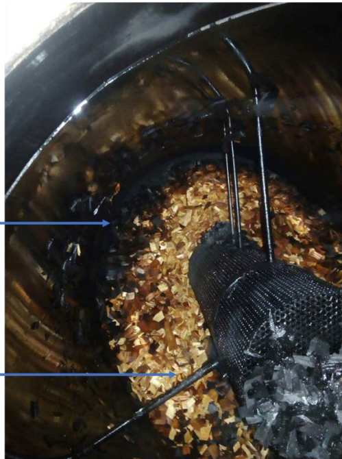
Figure 5.2: View of the wood chips in the reactor for the test run after the top layer of 3 cm had been removed.
