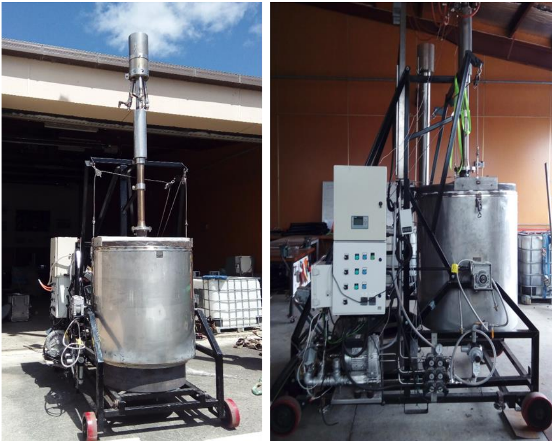
Figure 3.1: Massey 60 kg reactor front and side view
