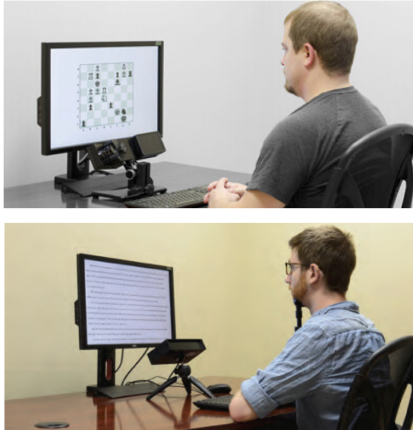
Figure 2.1: Examples of screen-based eye trackers. Top image is the EyeLink 1000 Plus device by SR Research. Bottom image is the EyeLink Portable Duo device by SR Research [1].
