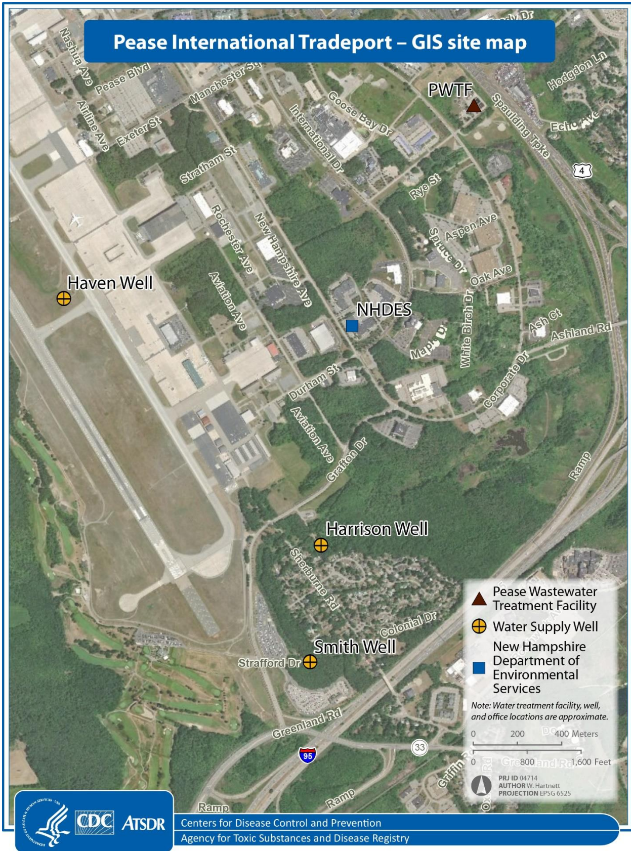
Figure A-3. Location of the Pease International Tradeport public water supply wells
