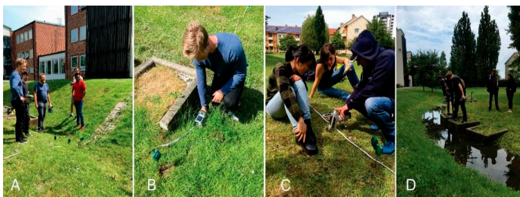
Figure 4. Quick scan mapping with portable XRF (X-ray fluorescence) measuring content of potential toxic elements in the topsoil of a swale. Here students are demonstrating measurements along a profile across the swale. Profiles are collected in the swale (A), covering the inlets (B), the deepest part (C), and the outlet of the swale. (D) shows the swale filled with rainwater and infiltration of surface water into the ground.
