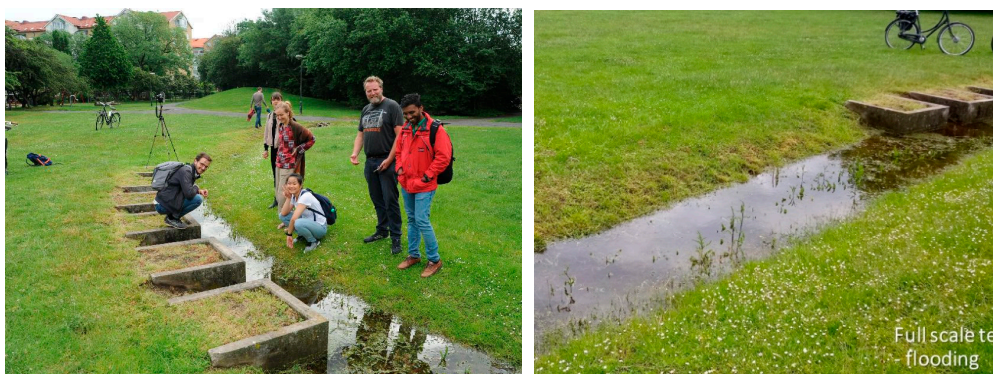
Figure 6. Discussion during monitoring in the swale in Augustenborg (left). Dataloggers were placed at several locations in the water (right) and time-lapse photography recorded the infiltration process.
