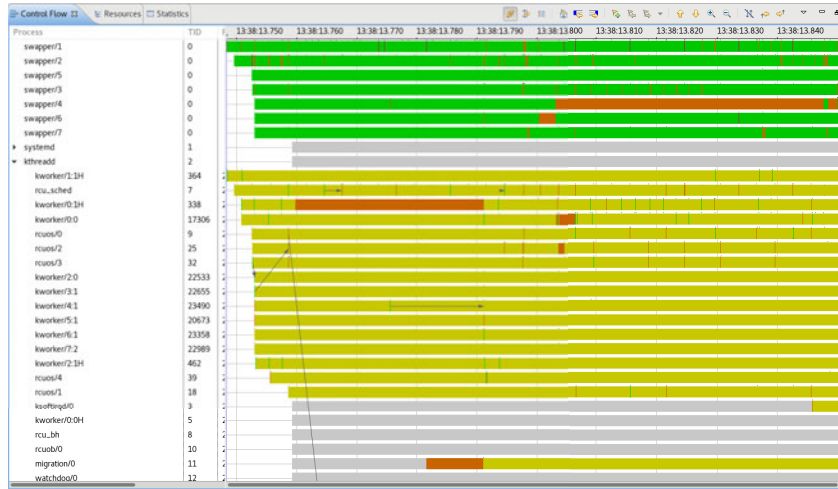
Fig. 13: The Control Flow View, a Time Graph View in Trace Compass
