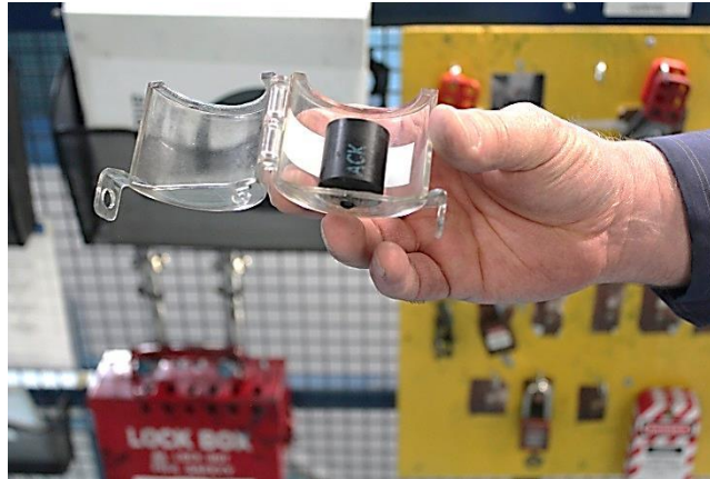
Figure 4-4 Pad-lockable cap to an emergency stop button
