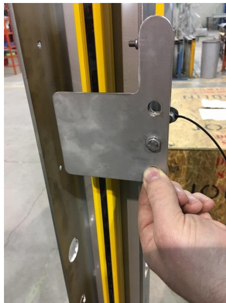
Figure 4-3 Safety curtain that could be locked in the activated position
