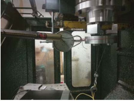
Figure 7: Lateral stiffness measurement by manual lateral force measurement with spring balance.
