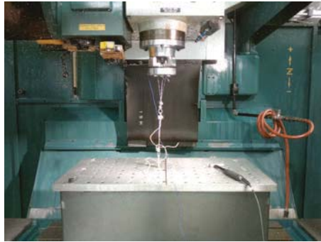
Figure 11: A 5 mm gap between the master and slave is maintained by a string arrangement.
